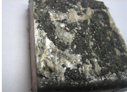
Photo of severe spark Erosion Damage.
