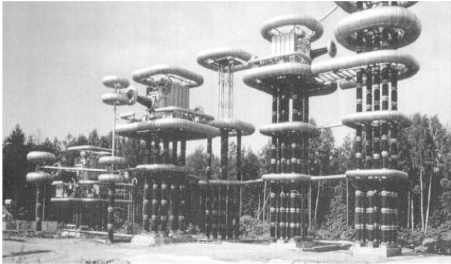
fig.2. Cascaded testing transformers with metal tanks and coolers Total voltage 3000 kV, 4A (courtesy HIGH-VOLT Dresden, Germany)
