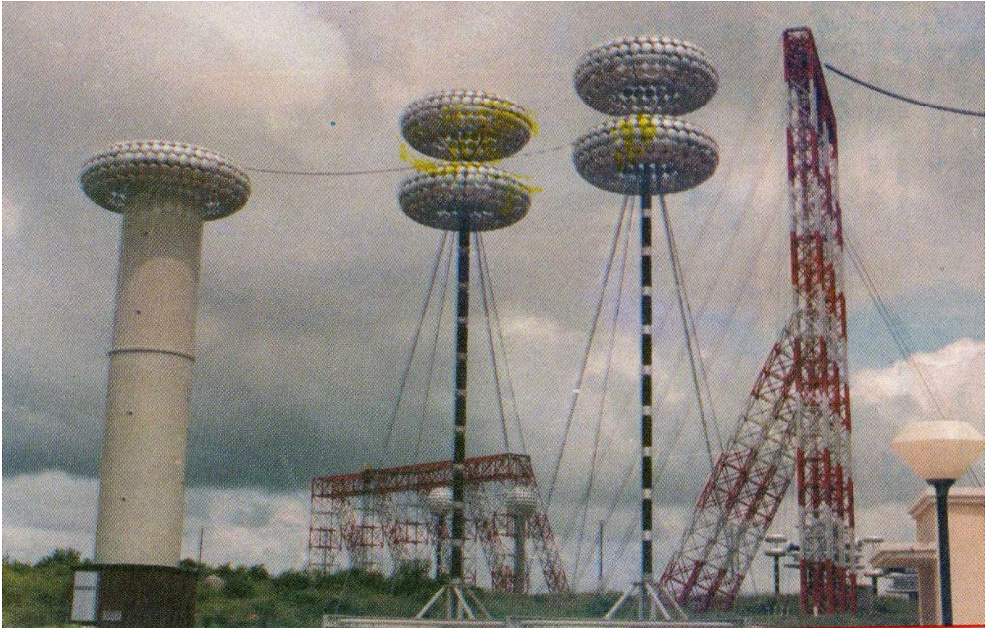
fig.25 5 MV, 500 kJ, Outdoor Type Impulse Generator with Capacitor Divider & Loading Capacitor
