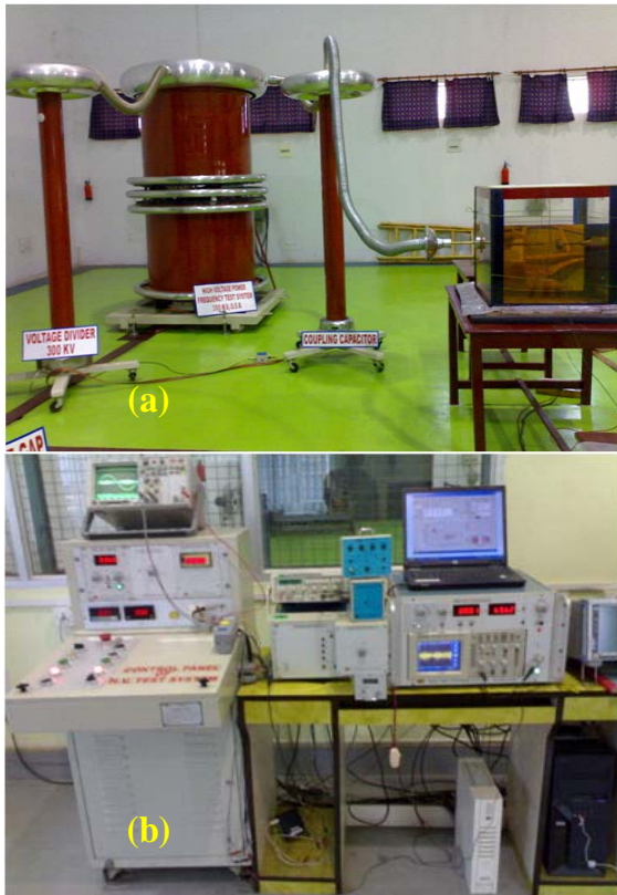
Fig. 1 Experimental setup for partial discharge test in ICTRHVL
