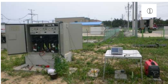
Figure 3: KEPCO's field test yard and Artificial Fault Generator (1)
