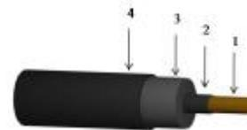
**Figure 1:** The coaxial insulation system, (1) Conductor, (2) Inner semicon layer, (3) Polymer insulation (XLPE), (4) Outer semicon layer.
