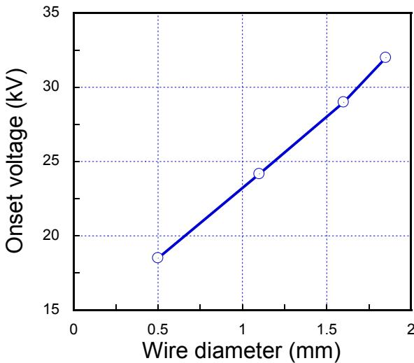
**Figure 3:** Dependence of corona onset voltage on wire diameter
