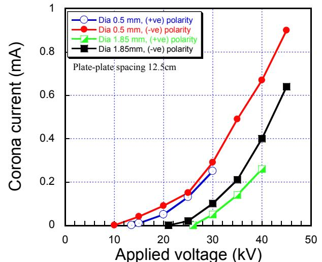
**Figure 2:** Effect of voltage polarity on precipitator corona current
