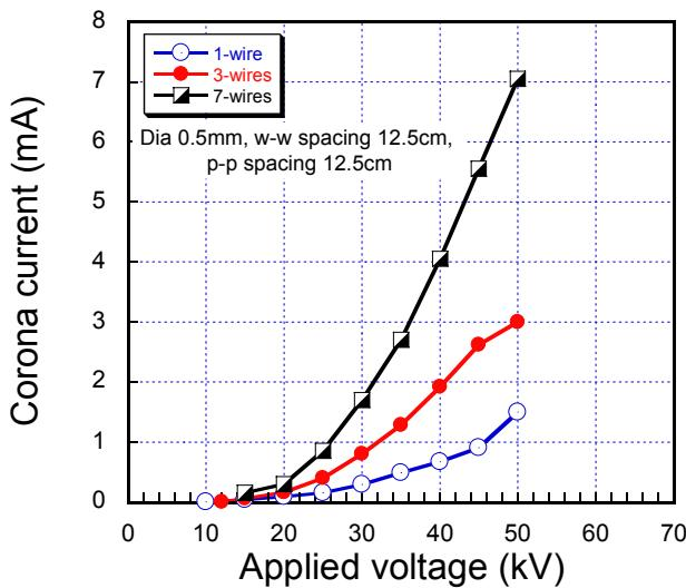
**Figure 5:** Effect of number of discharge wires on precipitator corona current
