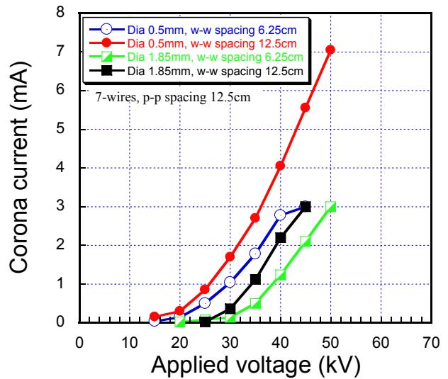
**Figure 7:** Effect of wire diameter on precipitator corona current (in case of 7-wires)
