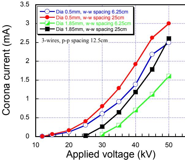
**Figure 6:** Effect of wire diameter on precipitator corona current (in case of 3-wires)
