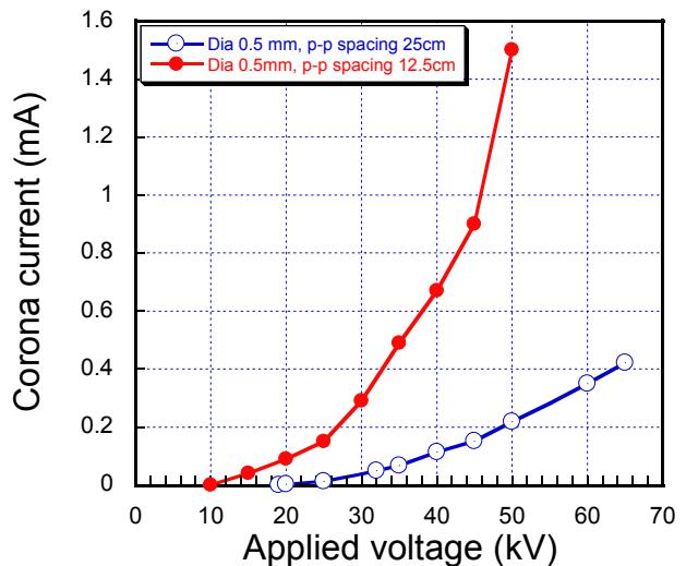
**Figure 4:** Effect of spacing between grounded plates on precipitator corona current
