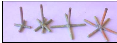
Figure 12: Configuration of rods used as scale model for the effect of Number of Rod Radial (N) and Radial Length (RL)
