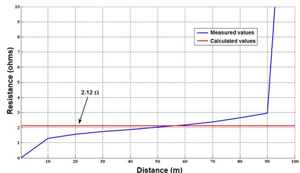
**Figure 6:** Curve of ground resistance versus distance
