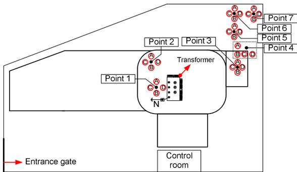
**Figure 4:** Step voltage measurement scheme
