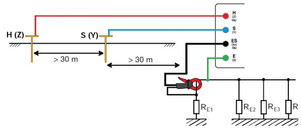
**Figure 1:** Configuration of the grounding grid resistance measurement procedure
