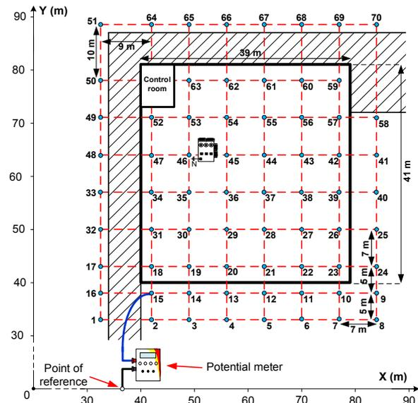
**Figure 8:** Sketch of the land area of the substation which was used to measure the surface potential
