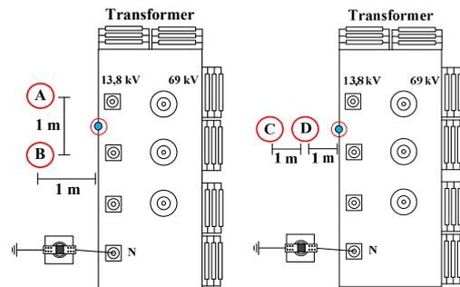
**Figure 3:** Measurement scheme of the touch voltage on the transformer housing
