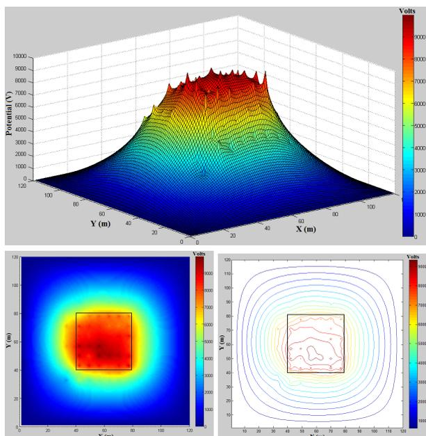
**Figure 9:** Behavior of the levels of superficial potential in the occurrence of a short circuit
