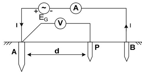
**Figure 5:** Scheme for measuring ground resistance with the grid de-energized
