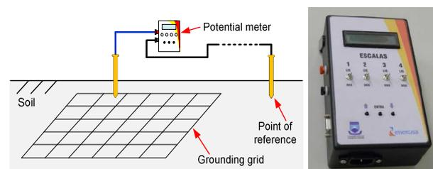
**Figure 2:** Measuring scheme and photograph of the surface potential meter
