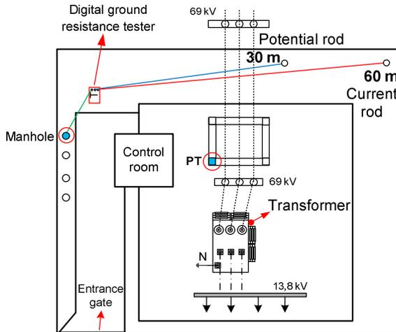
**Figure 7:** Sketch of the scheme for measuring the grounding grid resistance at the energized substation
