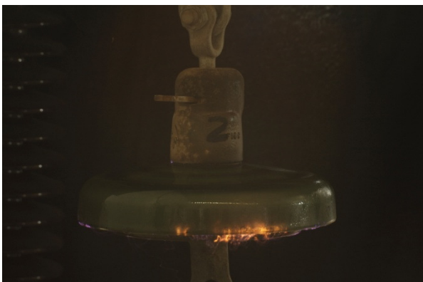
Figure 10: Recorded image of wet flashover.
