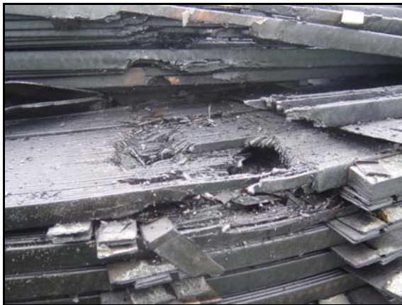
Figure 1 Failure of transformer by shorted turns
