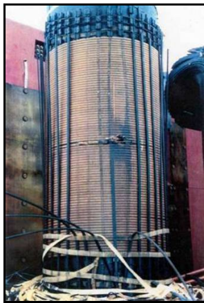
Figure 3 LV winding fault caused by overheating
