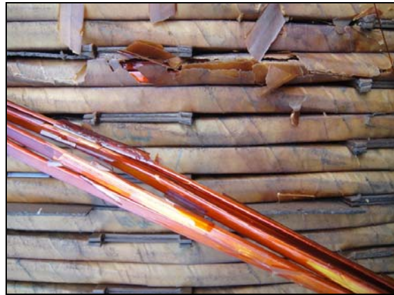
Figure 2 Developed hotspots on LV winding
