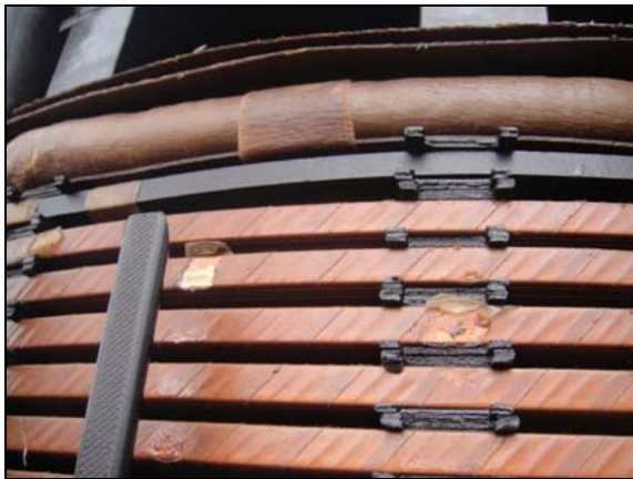
Figure 5 Understanding the implication of increasing risk of failure: LV winding failure in 2002 (up) and LV winding mechanical damage found in sister unit in April 2010 (down)
