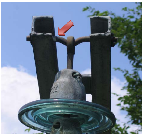
Figure 5: Arcing damage at a cross arm of a 20kV Line.
