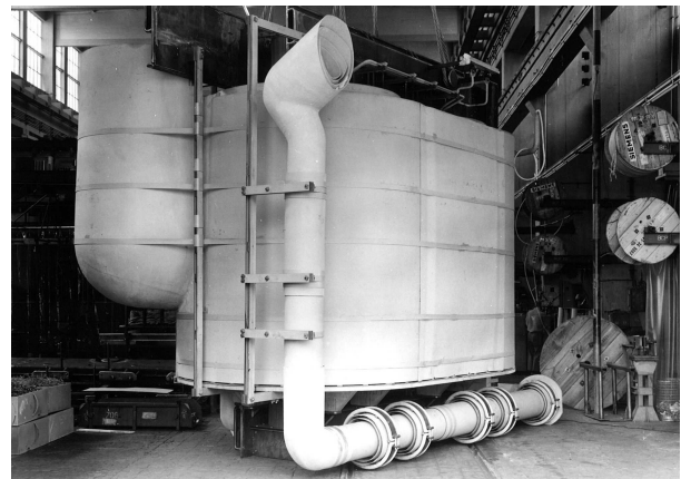
Figure 2: Active part of the 1200 kV prototype transformer
