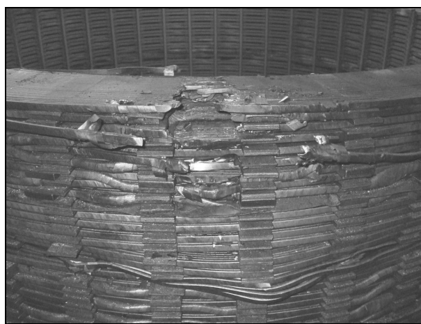
Figure 6: Damage to Series Winding, case study 5
