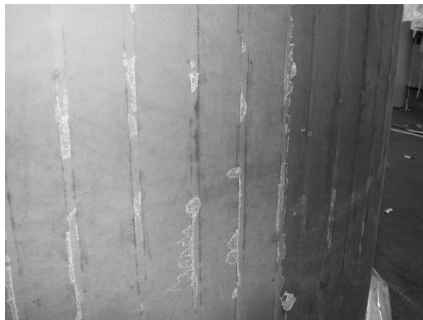
Figure 2: Partial Discharge Damage, case study 3
