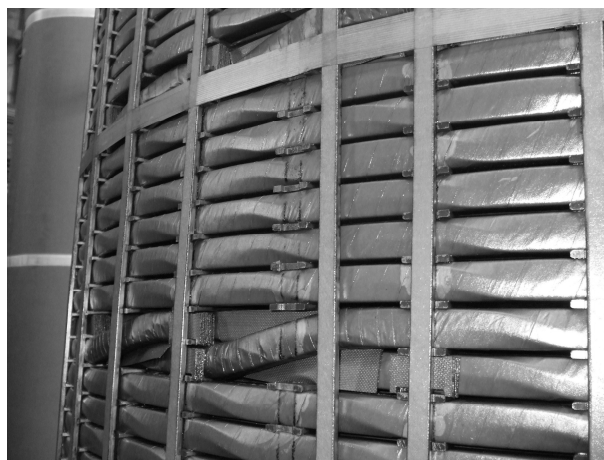
Figure 3: Partial Discharge Damage, case study 2
