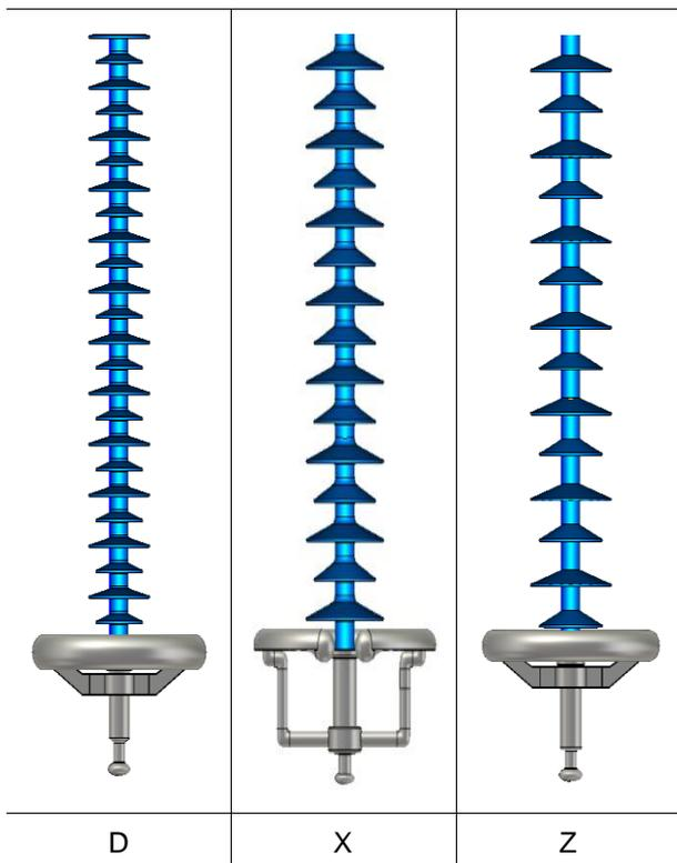
Figure 4: Polymer insulators design
