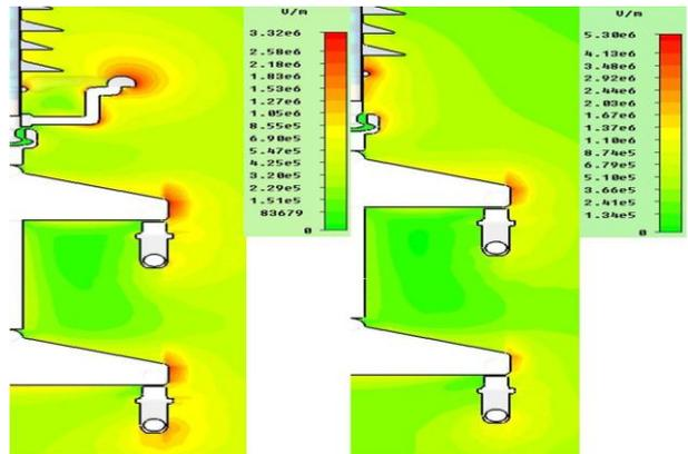
Figure 14: Geometry and contours for insulator end fitting (manufacturer X)
