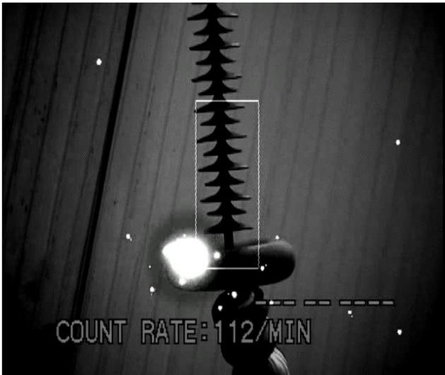
Figure 2: Correct position of corona ring
