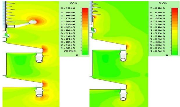
Figure 13: Geometry and contours for insulator end fitting (manufacturer D)
