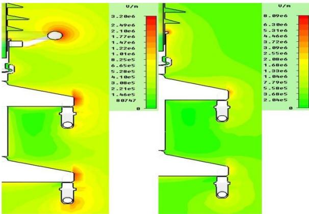
**Figure 15: Geometry and contours for insulator end fitting (manufacturer Z)**
