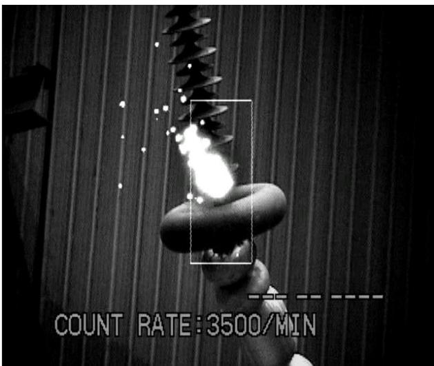
Figure 3: Incorrect corona ring position (2cm below of correct position)
