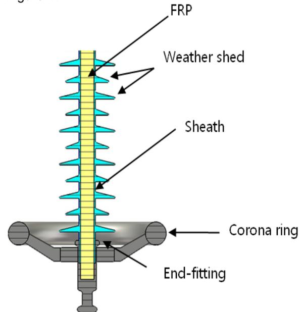
Figure 1: General outer shape of polymer insulator (manufacturer D)
