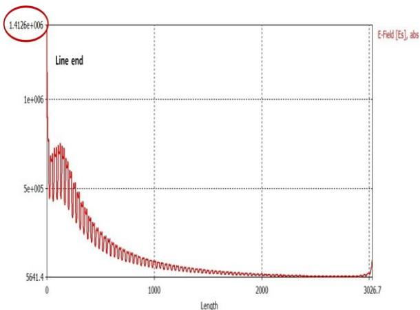
Figure 5: E-field distribution along the insulator surface (FDTD 3D)
