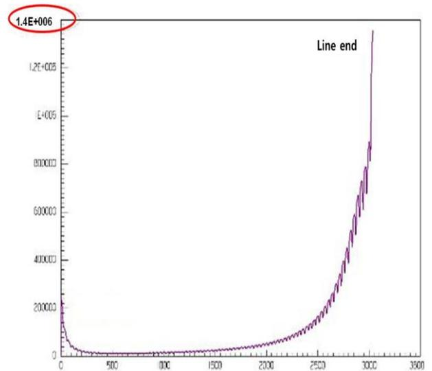
Figure 6: E-field distribution along the insulator surface (FEM 2D)
