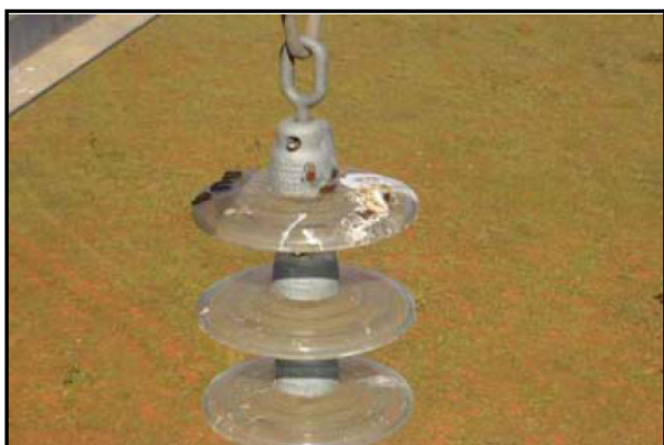
Figure 5: Curicaca's droppings on 69 kV TL insulator surface [5]
