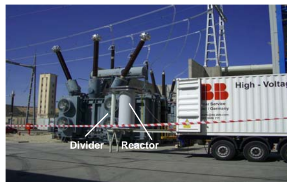
Figure 5: AC HV-Test on site on a 400kV transformer
