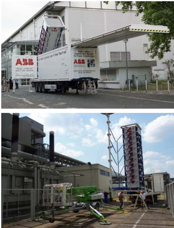
Figure 6: Impulse test on a 600MVA/400kV GSU
