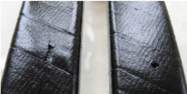
Figure 6: Surface of a specimen from group B with the puncture after the breakdown
