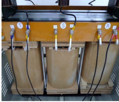
Figure 4: The arrangement of windings in model transformer.
