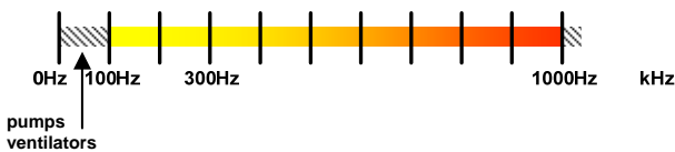
Figure 2: Frequency spectrum of transformer vibrations
