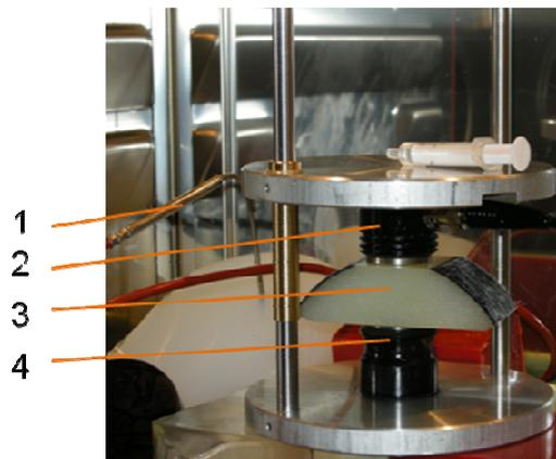
Figure 1: Test equipment for measurement of acoustic characteristics located in a temperature chamber ( $-20$  °C till  $+50$  °C) for a frequency range from 200 kHz till 600 kHz.
