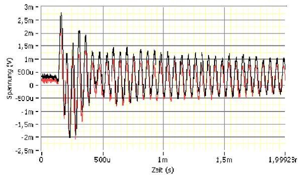
Figure 4: Sensor signal responses from two different excitations to prove the sensor reproducibility.
