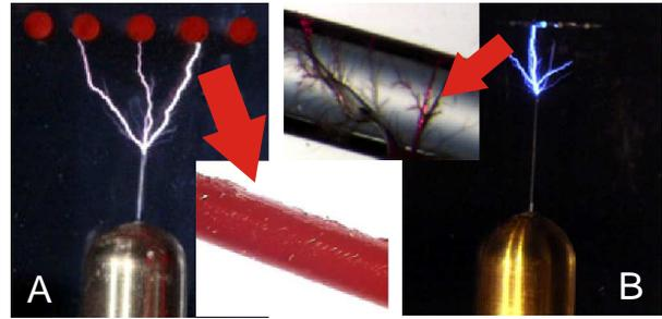
Figure 7: PDs on fluorescent silicone fibre-like samples (A), PMMA fibres (B); microscopic pictures (central) of the fibres after being exposed to trees.
