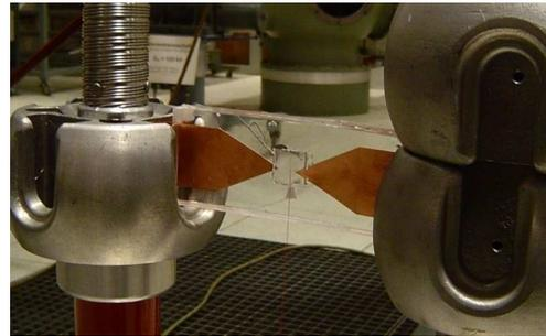
Figure 5: Silicone sample with embedded sensor prepared for measurement of PD signals.
