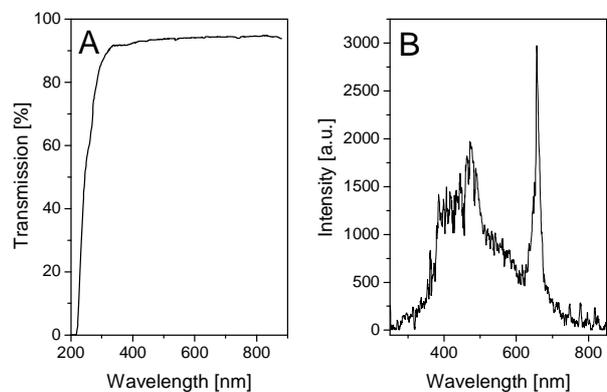
Figure 6: Wavelength depending transmission of a 10 mm layer of silicone (A), and spectrum of PD in silicone (B), both Elastosil 7665.
