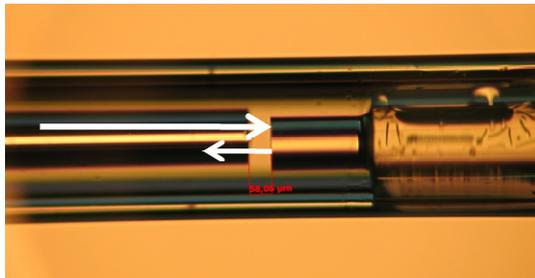
Figure 2: Above: Scheme of the used fibre Fabry-Perot acoustic sensor; below: designed sensor sample for experimental investigation in HV environment.
