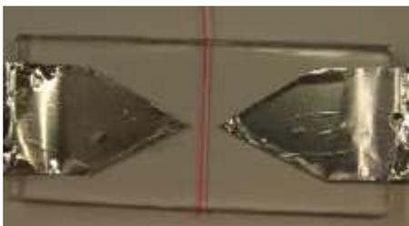
Figure 9: Sample with fluorescent optical fibre (PMMA) embedded between two Aluminium electrodes (Silicone: Elastosil RT 604).
