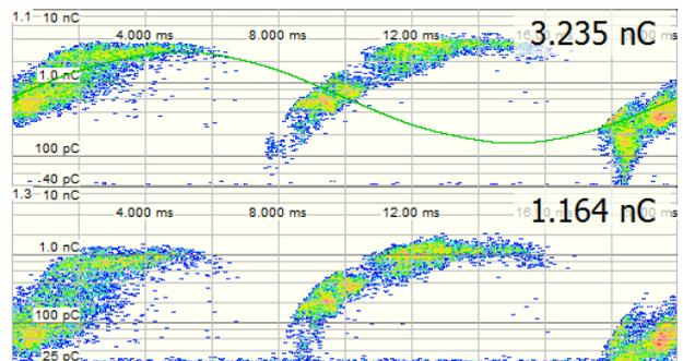
Figure 8: PRPD pattern (electrical channel above, optical channel below), cable and tip in air on high AC voltage of 19 kV.
