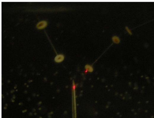
Figure 3: EFPI sensor samples embedded in transparent silicone elastomer, radially aligned to the needle under high voltage. (The illuminated points come from the laser beam.)
