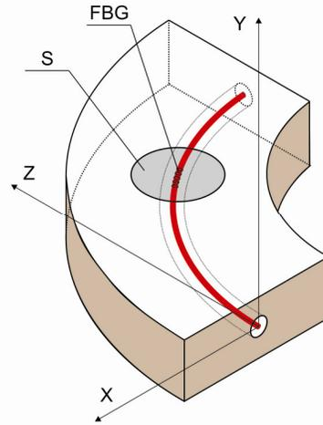
**Figure 2:** FBG embedded in the pressing ring. Z - the longitudinal direction; X, Y - the transverse directions; Y - the direction on which the pressing force is applied
