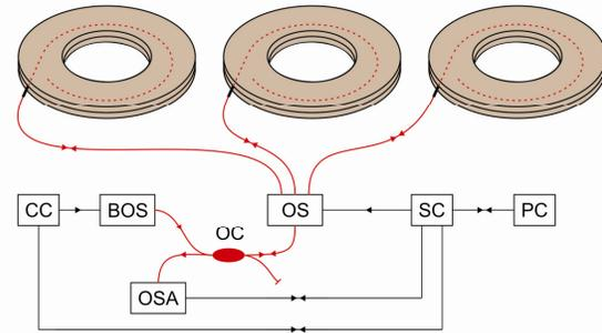
**Figure 4:** Principle diagram of the axial forces measuring system at a power transformer with smart pressing rings. OS - optical switch 1x3, OC - optical coupler 2x2, OSA - optical spectrum analyzer, SC - system controller, CC - current controller, BOS - broadband optical source, PC - computer, — FO link, — electrical link.
