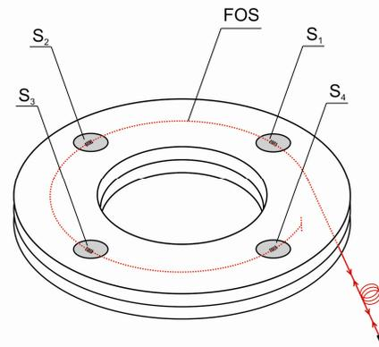
**Figure 1:** Top view of a smart pressing ring S1, S2, S3, S4 - areas where the controlled axial clamping is achieved, FOS- quasi-distributed strain sensitive FBG optical sensor
