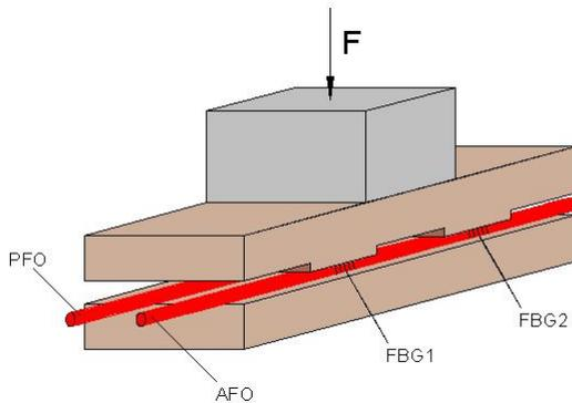
**Figure 3:** Experimental device for determining the FBG sensor transverse strain sensitivity. AFO-active FO, PFO- passive FO
