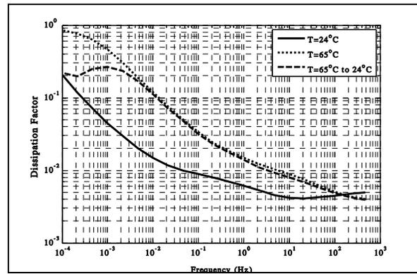
**Figure 9.** Effect of temperature transition on dissipation factor.
