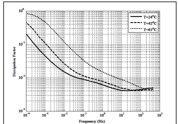
**Figure 5.** Effect of temperature on dissipation factor.
