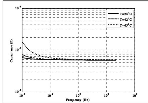
**Figure 4.** Effect of temperature on capacitance value.
