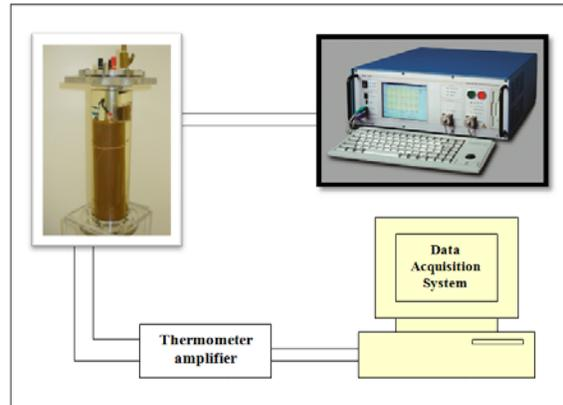
Figure 3. Test arrangement for the FDS and temperature measuring
