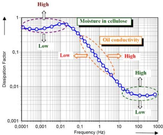
Figure 2. Separate impacts of oil conductivity and moisture in cellulose on Frequency Domain Spectroscopy (FDS).
