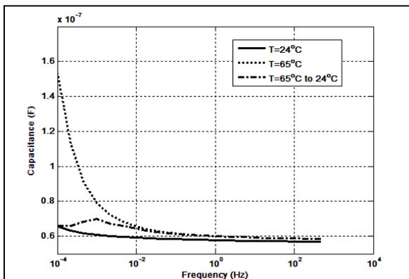
**Figure 8.** Effect of temperature transition on capacitance value.
