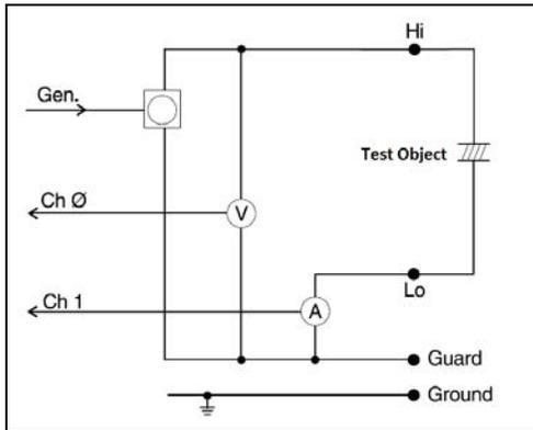
Figure 1. Schematic block diagram of the IDA 200-system measurement
