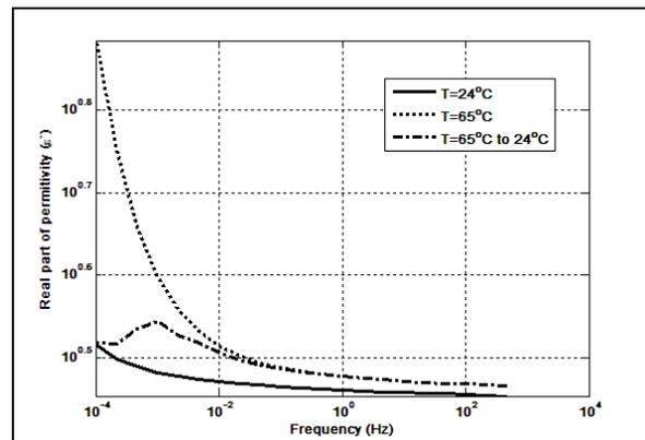
**Figure 10.** Effect of temperature transition on real part of permittivity.
