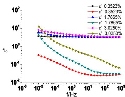
**Fig 9:** Complex permittivity spectroscopy of insulation pressboard with different water content.
