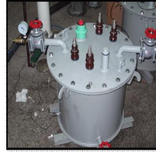
**Fig 3:** Model transformer with alternative geometric structure of main insulation
