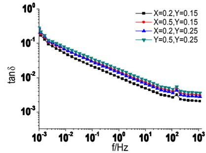
**Fig 5:** Influence of geometry on dissipation factor spectroscopy of oil paper insulation system with the lower conductivity oil ( $\sigma = 0.01\text{pS/m}$ ) .
