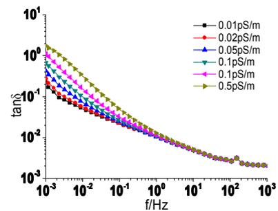
**Fig 7:** Influence of oil conductivity on dissipation factor spectroscopy of oil paper insulation system with the lower conductivity oil.
