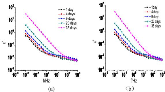
**Fig 12:** Complex permittivity spectroscopy of oil impregnated pressboard with different aging level at 130°C. (a)  $\epsilon' - f$  (b)  $\epsilon'' - f$
