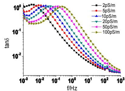
**Fig 8:** Influence of oil conductivity on dissipation factor spectroscopy of oil paper insulation system with the higher conductivity oil.
