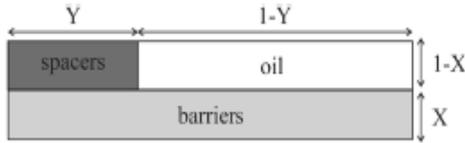
**Fig 2:** X-Y representation of transformer main insulation.
