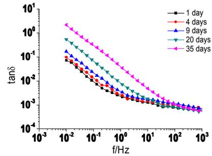
**Fig 13:** Dissipation factor spectroscopy of oil paper insulation with different aging level.
