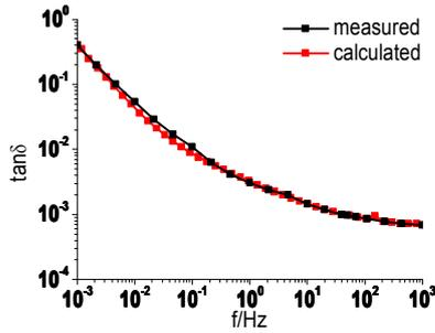
**Fig 4:** Comparison between simulation curve of X-Y model and onsite measured curve of transformer model
