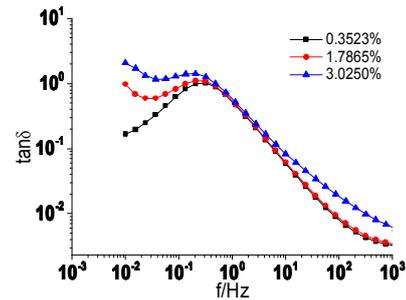
**Fig 11:** Dissipation factor spectroscopy of oil paper insulation with different water content with the higher conductivity oil ( $\sigma = 100\text{pS/m}$ ).
