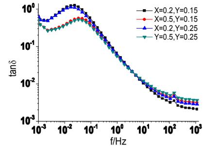
**Fig 6:** Influence of geometry on dissipation factor spectroscopy of oil paper insulation system with the higher conductivity oil ( $\sigma = 10\text{pS/m}$ ).
