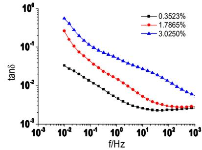
**Fig 10:** Dissipation factor spectroscopy of oil paper insulation with different water content with the lower conductivity oil ( $\sigma = 0.01\text{pS/m}$ ).
