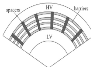
**Fig 1:** Section of main insulation in a core-type transformer.
