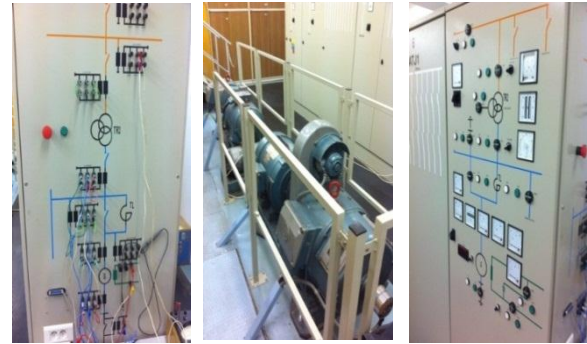
Figure 1: Physical model of power station – outputs from measurement transformers (left), synchronous generator and DC motor (middle), control panel (right)
