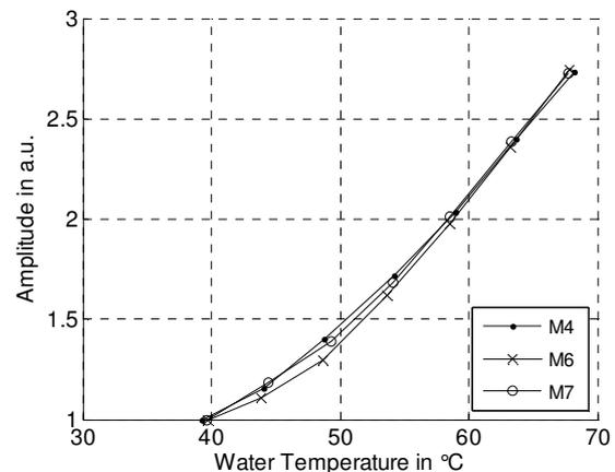
**Figure 8:** Maximum normalized ultrasonic amplitudes of the three ultrasonic measurements on sample type 1
