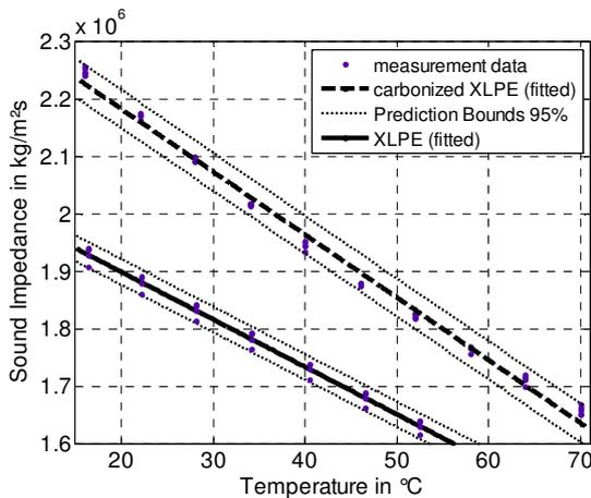
**Figure 3:** Sound impedances of XLPE and carbonized XLPE over temperature
