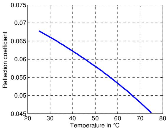
**Figure 4:** Calculated reflection coefficient of the interface between XLPE and carbonized XLPE dependent on interface temperature
