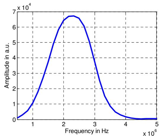
**Figure 2:** Frequency spectrum of a typical ultrasonic impulse
