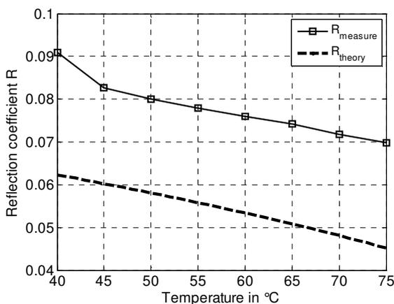
**Figure 10:** Reflection coefficient of the carbon interface over interface temperature, theoretical (dashed), measured (solid)
