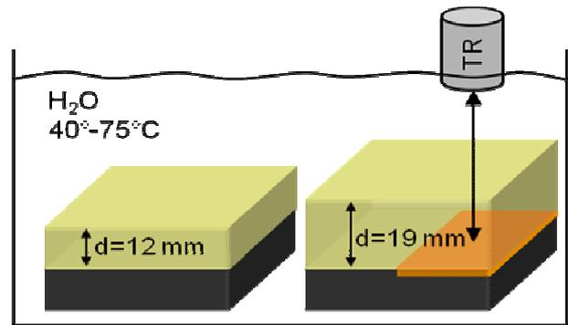
**Figure 7:** Test setup with synthetic samples, sample 1 with a carbon interface (left), sample 2 with metal reference (right)
