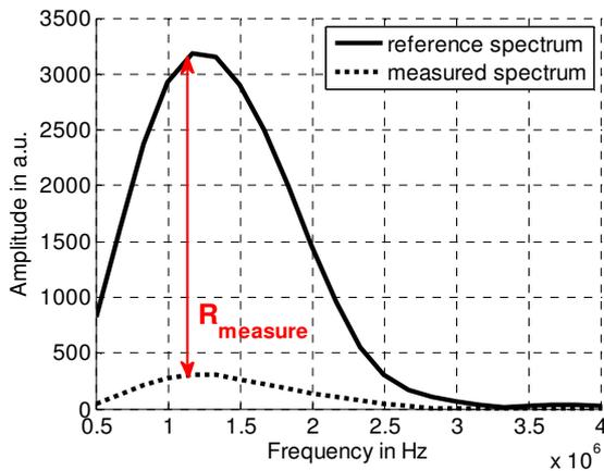
**Figure 6:** Comparison of signal spectrums to evaluate the reflection coefficient at a certain temperature
