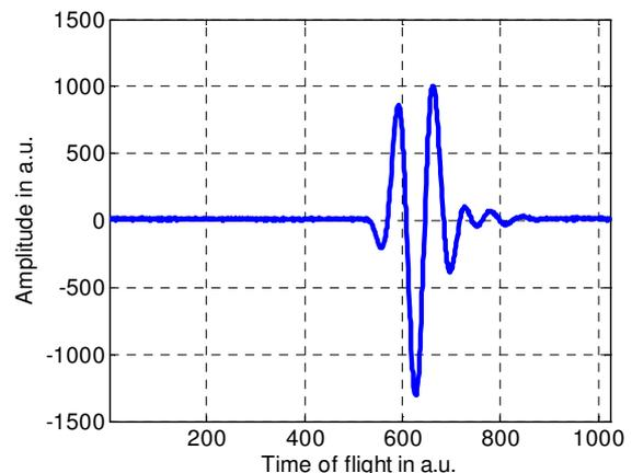
Figure 1: Typical ultrasonic impulse
