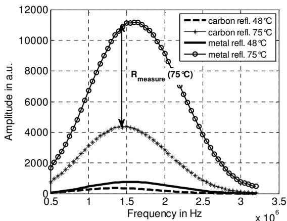
**Figure 9:** Exemplary frequency spectrums of the ultrasonic signals reflected at the metal interface and the carbon interface
