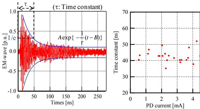
(a) Definition of attenuation time constant. (b) Measured time constant of EM-wave
