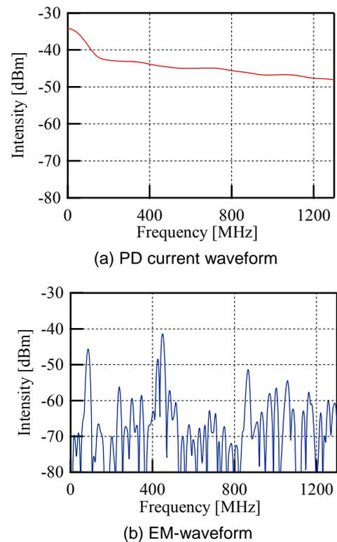
Figure 10 Frequency spectra of PD current and EM-waveforms ( $\phi 0.25$  mm,  $\ell = 5$  mm).
