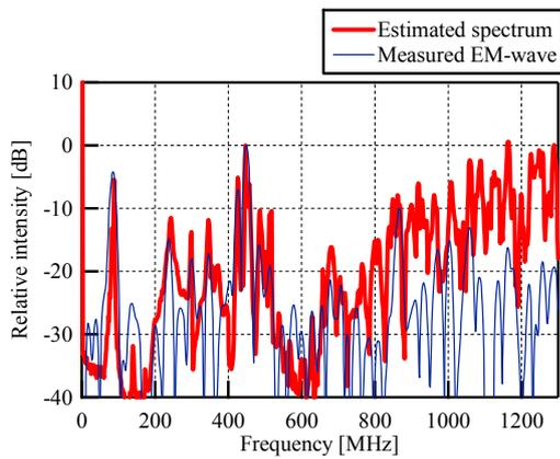
Figure 12 Comparison of estimated and measured EM-wave spectrum ( $\phi 0.25$  mm,  $\ell = 5$  mm).
