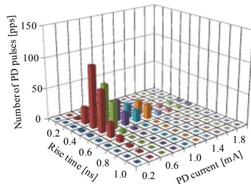
Figure 5 Distribution of the rise time and current of PD current pulses ( $\phi$  0.25 mm,  $\ell$  =3 mm).
