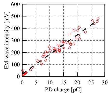
Figure 4 Correlation between charge of PD pulse and EM-wave intensity ( $\phi$  0.25 mm,  $\ell$  =10 mm).
