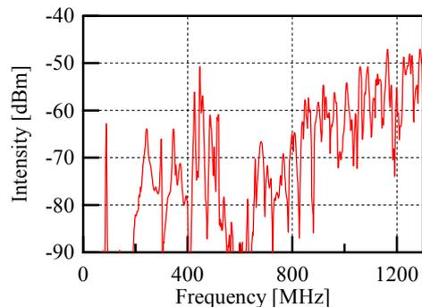
Figure 11 Propagation characteristics from particle to UHF sensor ( $\phi 0.25$  mm,  $\ell = 5$  mm).
