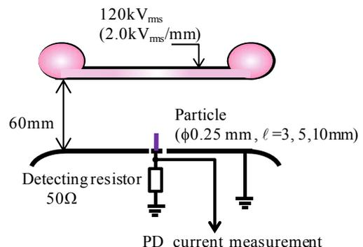
Figure 1 Electrode setup.
