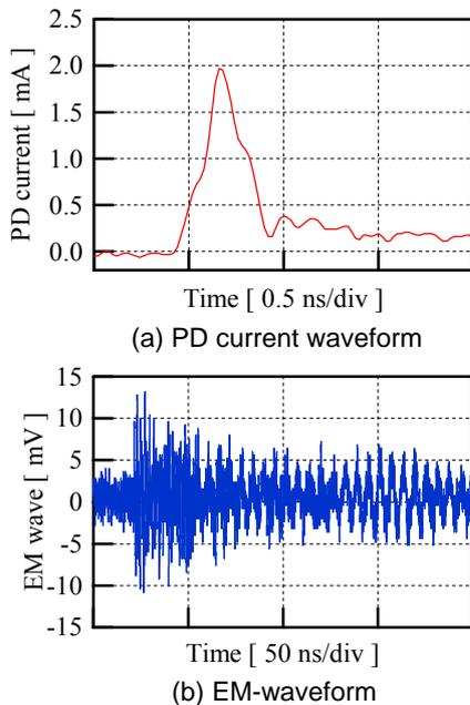
Figure 9 PD current and EM-waveforms ( $\phi 0.25$  mm,  $\ell = 5$  mm).
