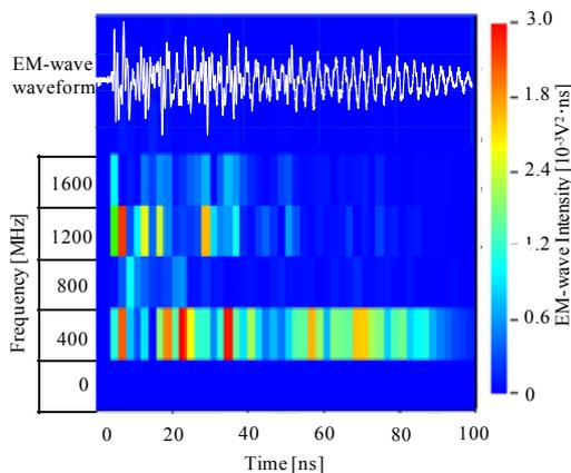
Figure 13 Sequential frequency characteristics of EM-waveform ( $\phi 0.25$  mm,  $\ell = 5$  mm).
