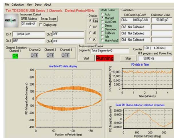
**Figure 4:** Typical snapshot of patterns acquired for Multiple Source PD
