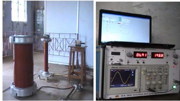
**Figure 2:** Typical Layout of Laboratory Setup and Digital PD Measurement and Acquisition System
