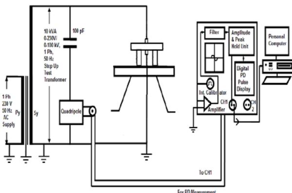
**Figure 1:** Generic Arrangement of PD Measurement and Acquisition System
