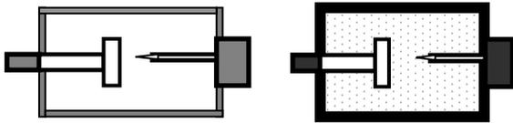
**Figure 4:** Laboratory models simulating Air and Oil Corona discharges
