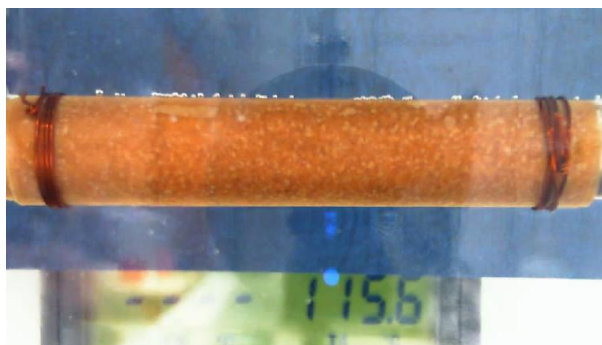
Figure 2: Paper - mineral oil, water content 5%, 115.6°C, start 92.2°C
