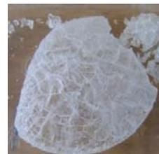
**Figure 3.2:** Silica Aerogel after drying
