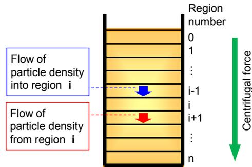
Figure 7: Calculation model of centrifuging process
