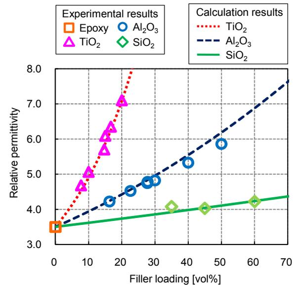
Figure 8: Relative permittivity of epoxy resin loaded with fillers
