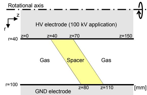
**Figure 1:** Calculation model for cone-type spacer
