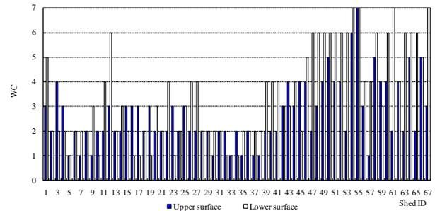
Figure 1. Hydrophobicity status of upper or lower surfaces of SR insulator sheds after years in service [7]
