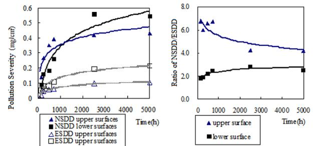
Figure 5. NSDD, ESDD and the ratio of NSDD/ESDD changing with time in Test 1-AC [4]
