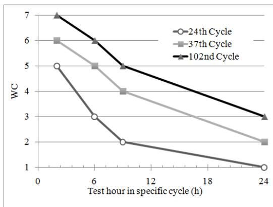
**Figure 7.** Hydrophobicity changes in different cycles. It takes more time for the insulator to recover to a better hydrophobicity status, such as WC2. Wettability class was measured at first sheds of grounded end of sample insulator  $B_L$  in Test I-AC [6].
