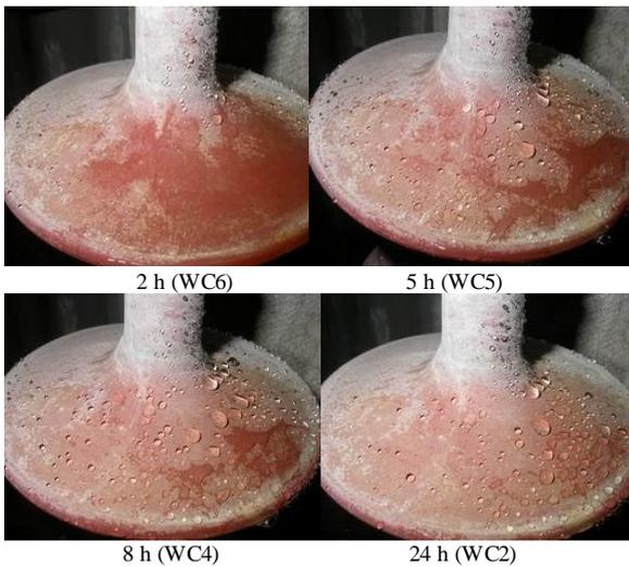
**Figure 6.** Hydrophobicity change due to transfer property in 24 h (in the UV chamber) at the 56th cycle of the test. First shed of grounded end,  $B_L$  in Test I-AC [6]
