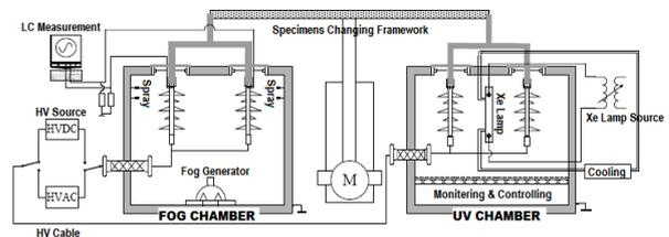
Figure 4. 5000 h multi-stress test equipment in Tsinghua University, with fog chamber and UV chamber separated.
