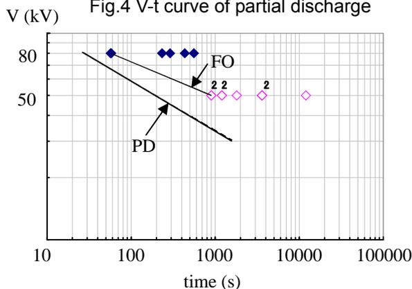
Fig.5 Comparison of V-t curve of partial discharge and creepage flashover
