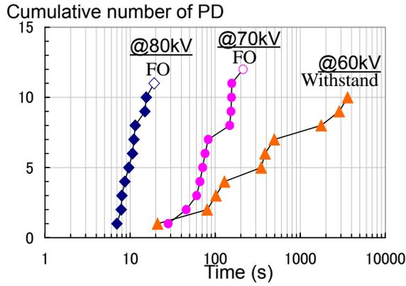
Fig.7 Dependence on applied voltage of cumulative number of PD and PD inception time occurred 10 times at 80 kV and FO occurred in approximately 20 seconds. At the 60kV, FO did not occur even after voltage was applied continuously for 1 hour.
