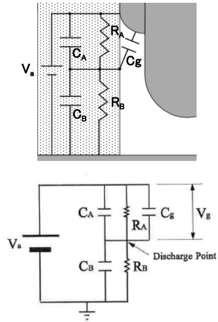
Fig.8 Equivalent circuit for PD at around a TJ circuit model for discharge point.
