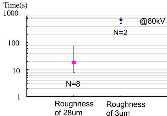
Fig.6 Dependence on surface roughness of FRP@80kV of PD inception time
