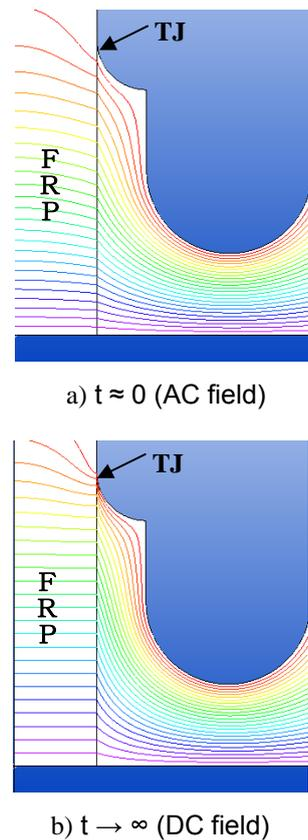
Fig.2 Equipotential line distribution
