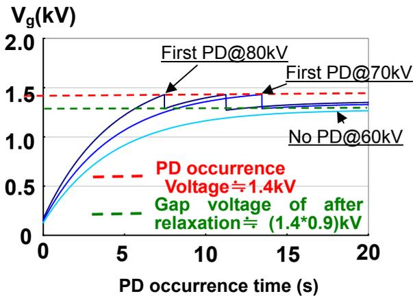
Fig.10 Results of calculation of equivalent circuit considered relaxation of electric fields near the TJ by PD.
