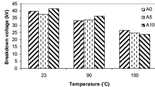
**Figure 1:** Histogram of breakdown voltage of samples vs. temperature
