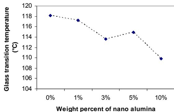
**Figure 1:** Glass transition temperatrue of cast epoxy systems vs. nano particle concentration
