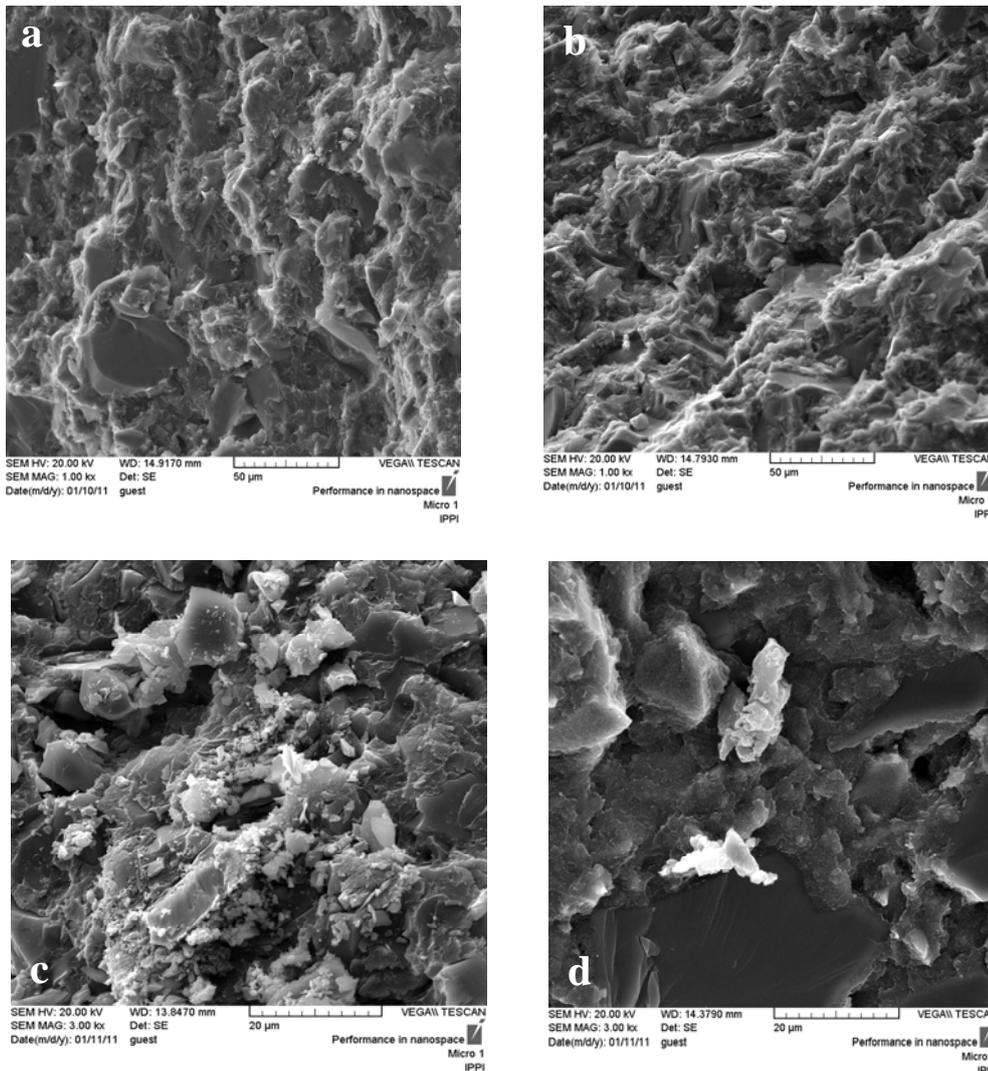
**Figure 4:** SEM micrographs of cast epoxy systems: a) A0 with magnification of 1000×; b) A1 (1000×); c) A5 (3000×); d) A10 (3000×).
