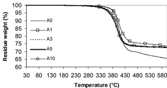
**Figure 3:** TGA curves of cast epoxy systems in the range of 30-600 °C
