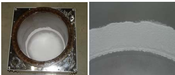
Figure 5: The picture of layer of SF 6 ice on the brim of inner cryostat : (a) SF 6 ice layer in the Dewar (b) Magnification of SF 6 ice layer
