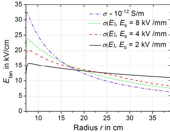
**Figure 2:** Distribution of the tangential electric field  $E_{\text{tan}}$  for the  $E$ - $J$ -characteristic curves shown in Figure 1 and for constant conductivity  $\sigma = 10^{-12}$  S/m
