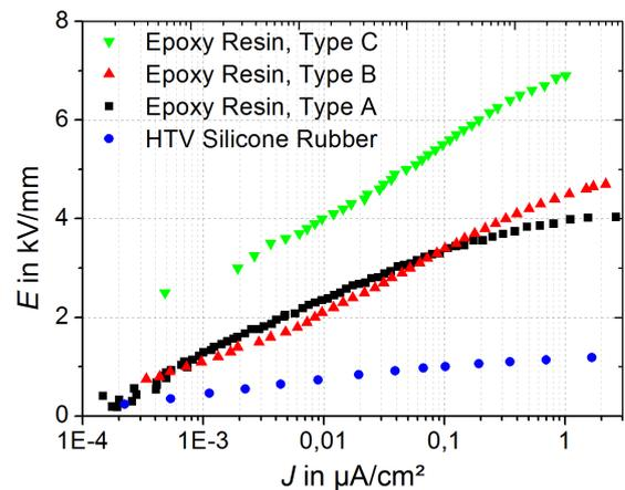
**Figure 4:** Measured  $E$ - $J$ -characteristic of the HTV silicone rubber and epoxy resin specimens
