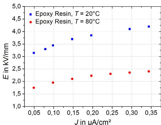
**Figure 6:** Temperature dependency of the  $E$ - $J$  characteristic for epoxy resin samples
