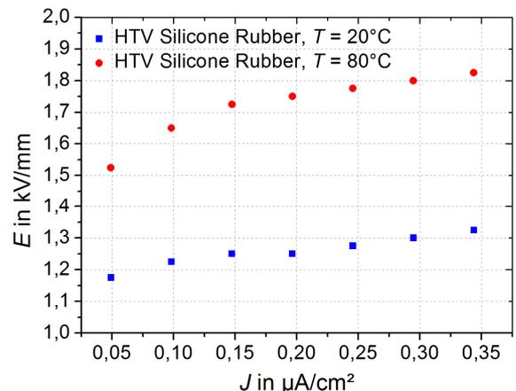
**Figure 5:** Temperature dependency of the  $E$ - $J$ -characteristic for HTV silicone rubber samples
