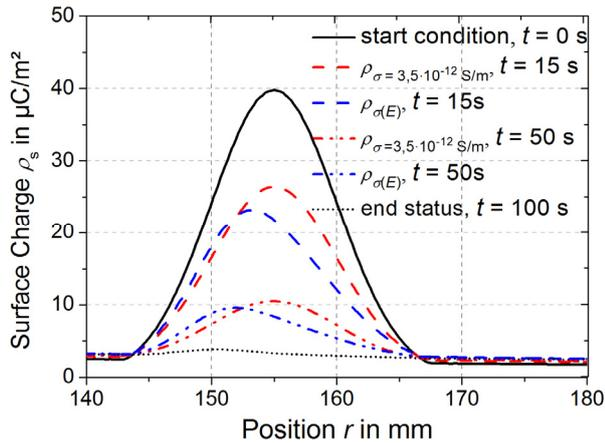
**Figure 3:** Surface charge flow-off characteristic of a linearly and a nonlinearly conductive insulator
