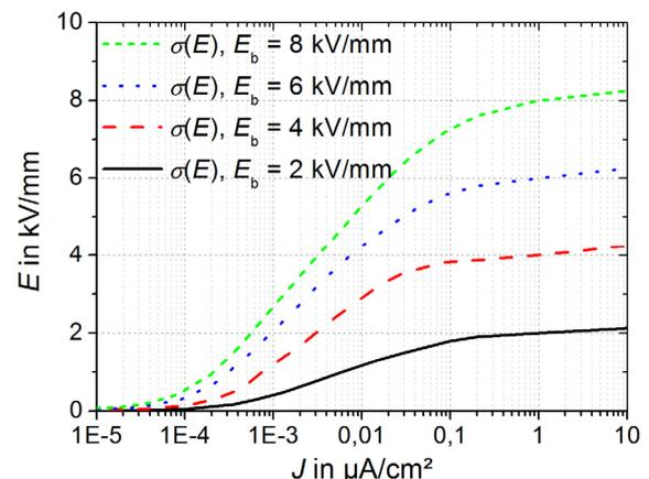
**Figure 1:** Nonlinear  $E$ - $J$ -curves used for the FEM simulation model
