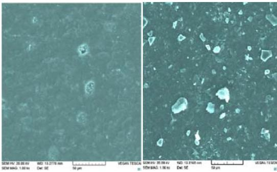
Figure 17: SEM analysis for aged and unaged SIR sample
