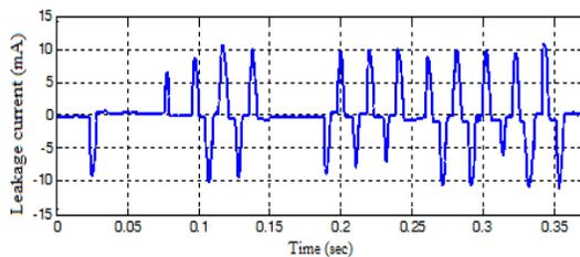
Figure 11: Leakage current of 20 kV polluted insulator contain fully formed arc with dry band arcing
