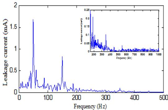
Figure 12: Frequency spectrum of Leakage current on 20 kV polluted insulator contain fully formed arcs with dry band arcing
