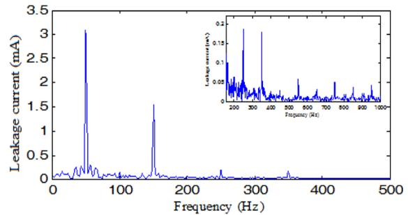
Figure 14: Frequency spectrum of Leakage current on 20 kV polluted insulator under UV contain fully formed arcs with dry band arcing
