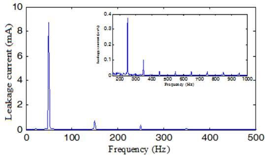
Figure 6: Frequency spectrum of Leakage current on 20 kV polluted insulator under UV
