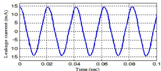
Figure 3: Leakage current of 20 kV polluted insulator
