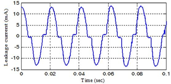
Figure 7: Leakage current of 20 kV polluted insulator contain dry band arcing
