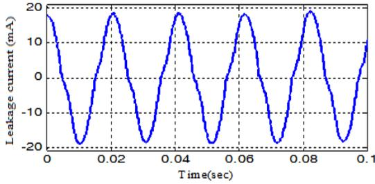
Figure 5: Leakage current of 20 kV polluted insulator Under UV
