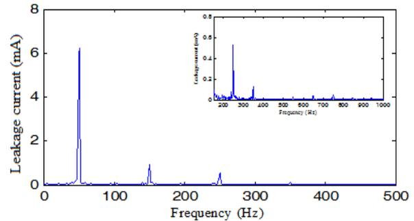
Figure 8: Frequency spectrum of Leakage current on 20 kV polluted insulator contain dry band arcing
