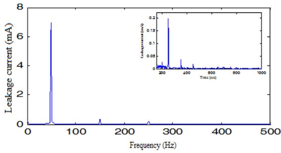
Figure 4: Frequency spectrum of Leakage current on 20 kV polluted insulator
