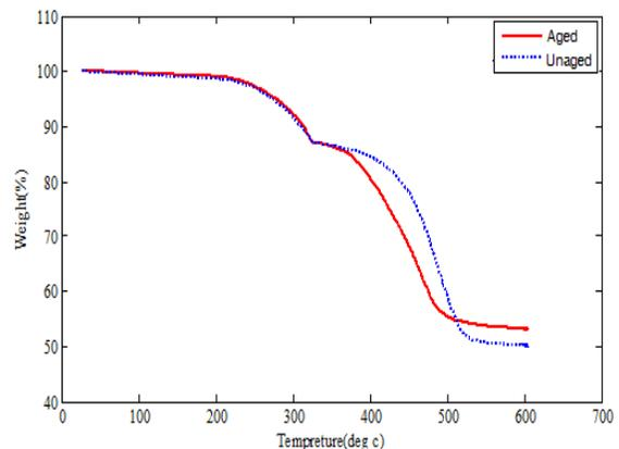
Figure 15: TGA analysis for aged and unaged polymer insulator
