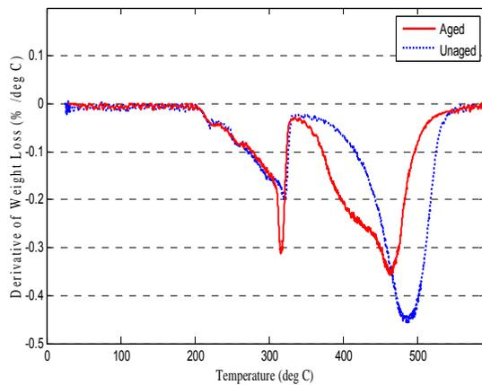
Figure 16: Derivative of Weight loss for aged and unaged polymer insulator
