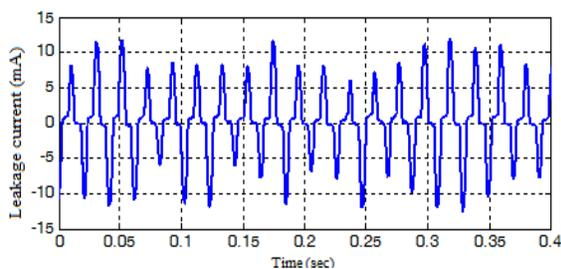
Figure 13: Frequency spectrum of Leakage current on 20 kV polluted insulator under UV contain fully formed arcs with dry band arcing
