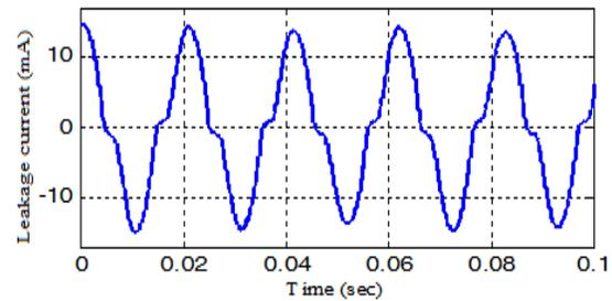
Figure 9: Leakage current of 20 kV polluted insulator under UV contain dry band arcing
