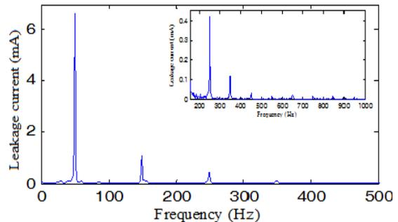
Figure 10: Frequency spectrum of Leakage current on 20 kV polluted insulator under UV contain dry band arcing
