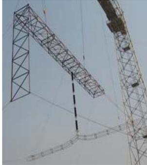
**Figure 6** Impulse voltage discharge experiment arrangement
