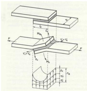
Figure 3: Stress distribution in a single-shear joint [3]
