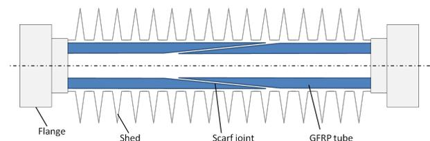
**Figure 1:** Principal assembly of an UHV insulator
