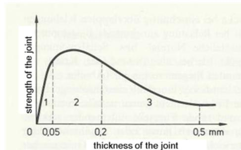
Figure 5: Joint strength as a function of the joint thickness [3]
