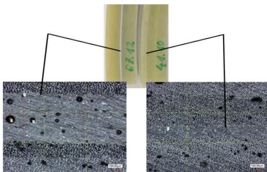
**Figure 14:** Microscopic investigation of two joints with different thicknesses [4]
