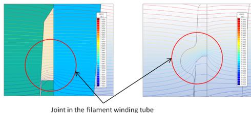
**Figure 11:** Equipotential plot in detail of the joint in the filament winding tube
