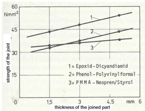
**Figure 7:** Joint strength as a function of the wall thickness of the parts [3]
