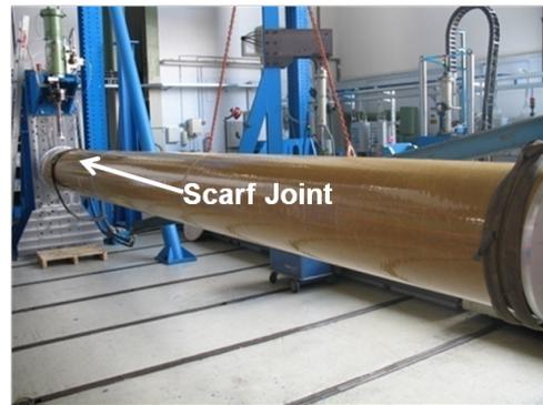
**Figure 16:** Setup for bending test
