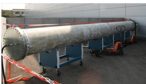
**Figure 15:** Setup for pressure test
