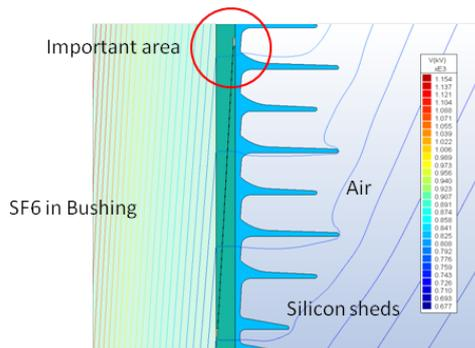
**Figure 10:** Equipotential plot of the joint in the filament winding tube
