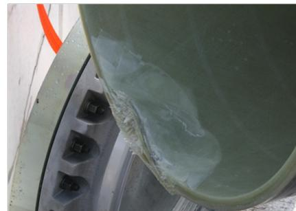
**Figure 17:** Failure during internal pressure test
