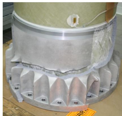
**Figure 18:** Failure during cantilever bending test
