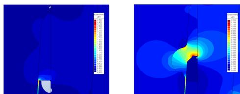
**Figure 12:** Field plot of the joint in the filament winding tube
