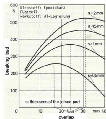
Figure 6: Joint strength as a function of the overlapping length [3]
