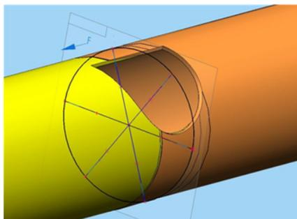
Figure 4: Scarf joint of two tubes
