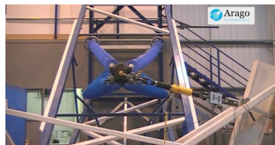
Figure 9: Failure containment: broken conductor test
