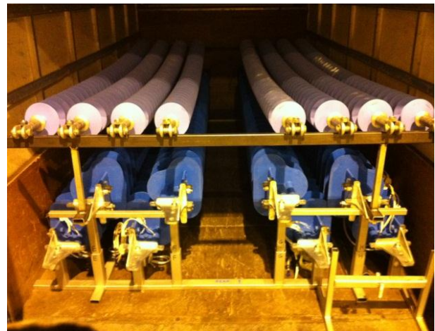
Figure 4: Four disassembled cross-arms en route to the installation site
