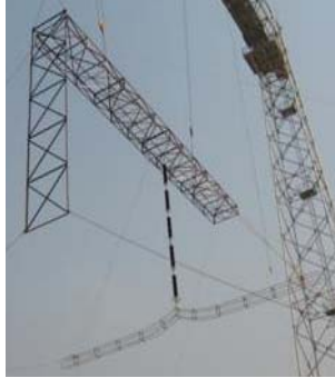
Figure 6 Impulse voltage discharge experiment arrangement
