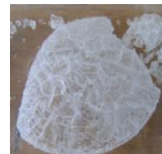
Figure 3.2: Silica Aerogel after drying
