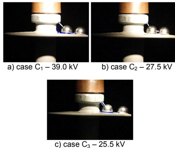
**Figure 3:** Corona in the semi-spheres.
