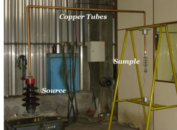
Figure 1: Overview of experimental setup.
