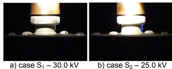
**Figure 4:** Corona in the water droplets.
