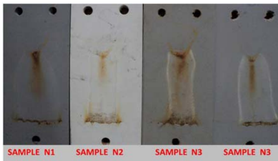
Figure 3: Photograph of samples with ATH nano filler subjected to IPTET+UV
