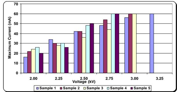
**Figure 14** – Maximum current during tracking test in samples with test composition 1
