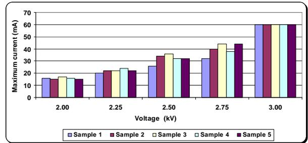
**Figure 15** – Maximum current during tracking test in samples with test composition 2
