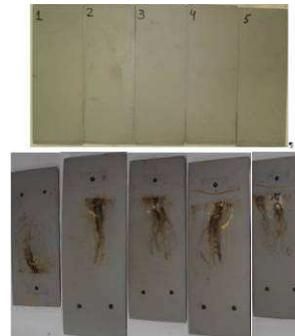
Figure 10 – TC 3 samples before and after tracking test
