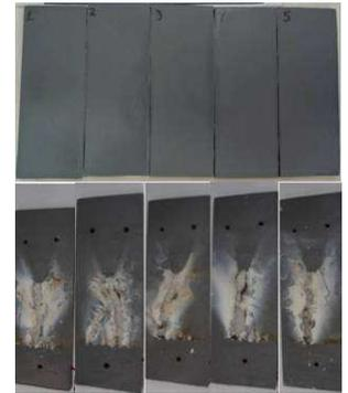
Figure 9 – TC 2 samples before and after tracking test
