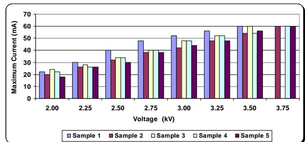
**Figure 16** – Maximum current during tracking test in samples with test composition 3
