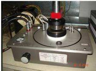
**Figure 1** – Tettex cell model 2914 for solid samples
