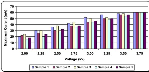
Figure 17 – Maximum current during tracking test in samples with test composition 4
