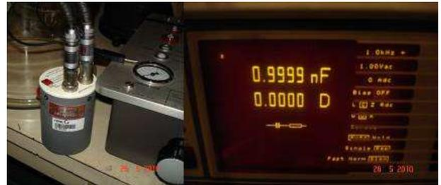
**Figure 4** - Standard Air capacitor type 1403-A, serial 6566 made by General Radio (1000pF ± 0.1%)
