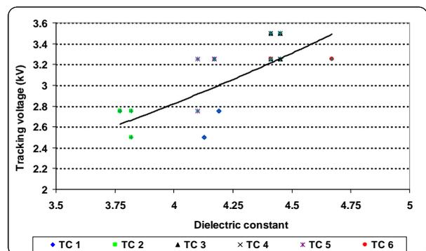
Figure 20 – Relationship between tracking voltage and dielectric constant
