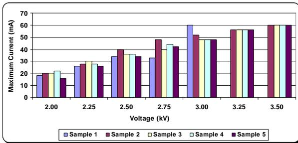
Figure 18 – Maximum current during tracking test in samples with test composition 5
