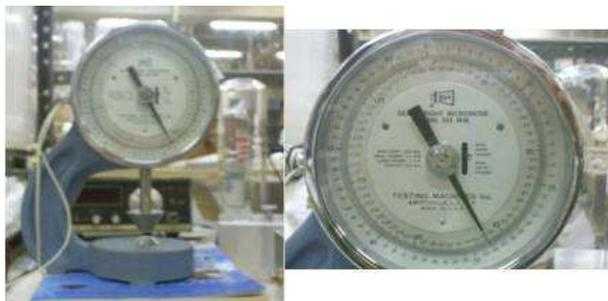
**Figure 3** - Dead Weight micrometer made by Testing Machines Inc, model 553 mm
