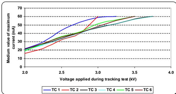
**Figure 22** – Variation of the current during tracking test
