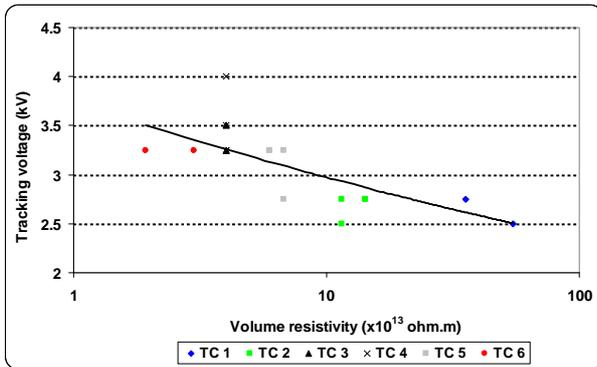
**Figure 21** – Relationship between tracking voltage and volume resistivity
