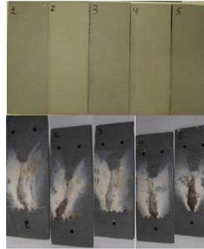
Figure 8 – TC 1 samples before and after tracking test
