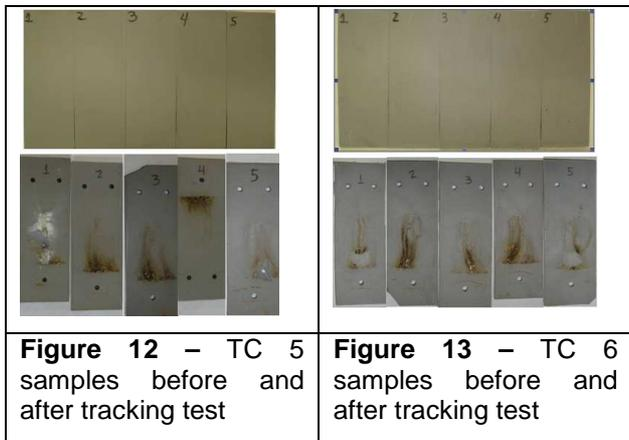
**Figure 12** – TC 5 samples before and after tracking test
