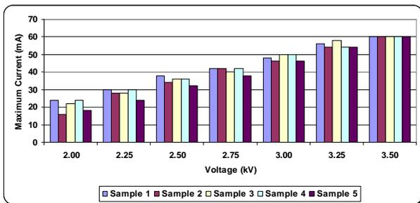
Figure 19 – Maximum current during tracking test in samples with test composition 6
