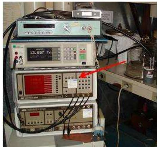
**Figure 5** - RLC bridge made by Wayne Kerr model 3245
