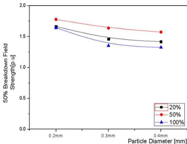
**Figure 18:** AC Test result for mixture ratio and particle diameter in same length
