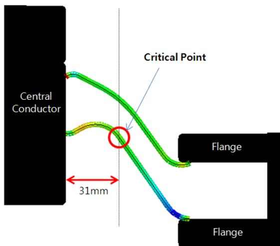
**Figure 7:** Analysis result for critical point of a particle
