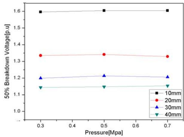
Figure 14: LI Test result for Pressure in 50%SF6 50%N2 gas
