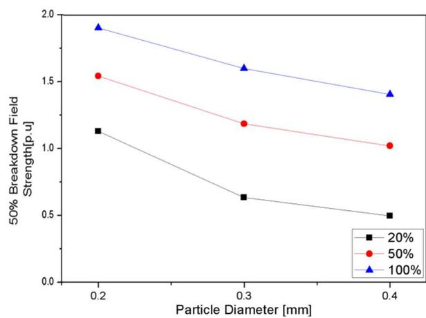
Figure 15: LI Test result for Particle Diameter in gas mixture ratio
