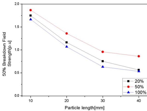
**Figure 16:** AC Test result for Particle length in gas mixture ratio
