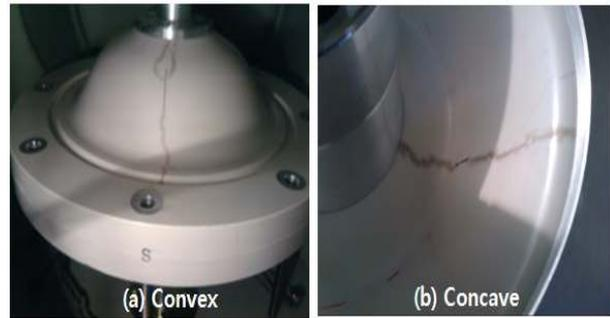
**Figure 8:** Breakdown picture of spacer for initial Tests
