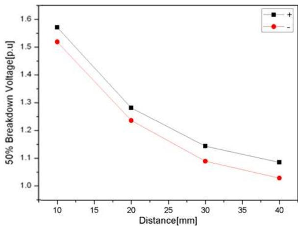
Figure 12: LI Test result for Polarity in 50%SF6 50%N2 gas
