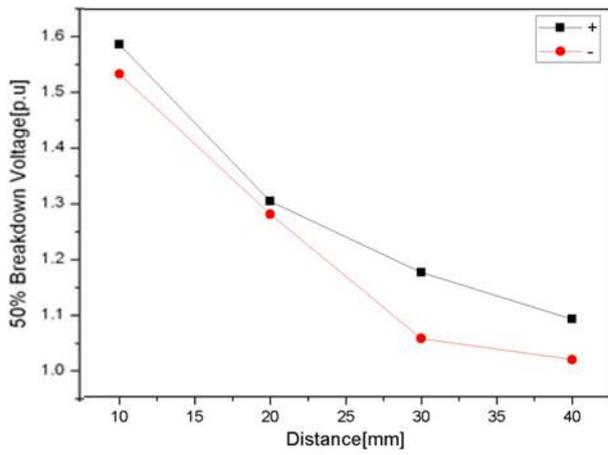
Figure 11: LI Test result for Polarity in 20%SF6 80%N2 gas
