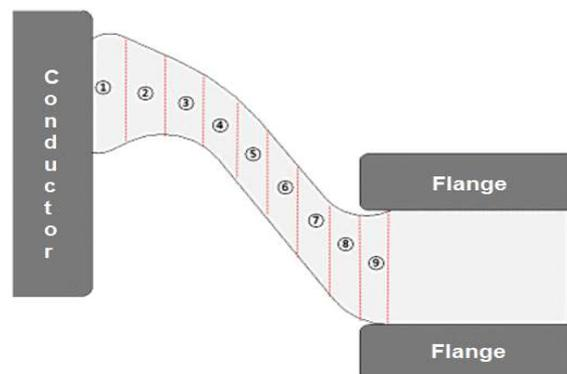
**Figure 5:** Spacer's surface attachment site for a particle
