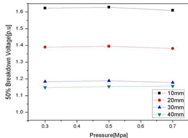
Figure 13: LI Test result for Pressure in 20%SF6 80%N2 gas
