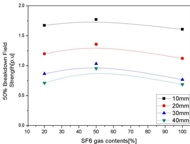
**Figure 17:** AC Test result for mixture ratio and particle length in same diameter's particle
