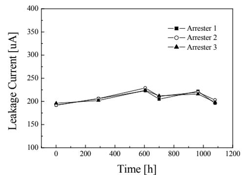
**Figure 3:** Variation of leakage current during tests.
