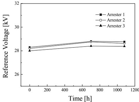
**Figure 4:** Variation of reference voltage during tests.
