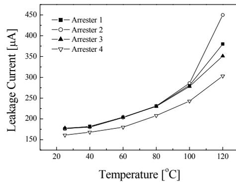
**Figure 5:** Leakage current with temperature.
