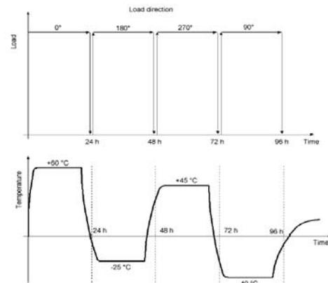
**Figure 2:** Cantilever load and temperature cycle of thermal mechanical test.
