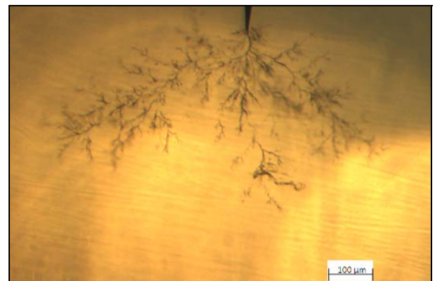
Figure 9: Treeing structures of neat epoxy (oEP) after exposure to 18 kV for 60 min
