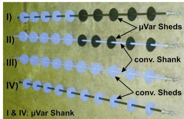
**Figure 2:** Example of four investigated insulators for  $U_m = 420 \text{ kV}$  [6]
