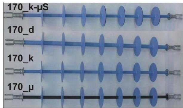
**Figure 5:** The four tested insulators
