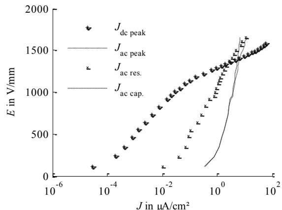
**Figure 1:**  $E-J$ -characteristic of the microvaristor filled silicone rubber separated in d.c. and a.c.
