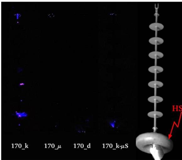
Figure 6: Different discharge-intensities on the four investigated insulators recorded at  $U_{d.c.} = 430$  kV and artificial rain (photography in the dark test hall; the daylight insulator photo on right hand side is for comparison and localization purposes)
