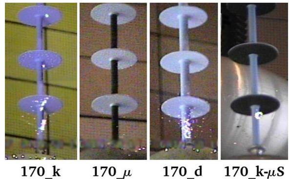
Figure 7: Different discharge-intensities at the four investigated insulators recorded at  $U_{d.c.} = 430$  kV and artificial rain with a UV daylight camera
