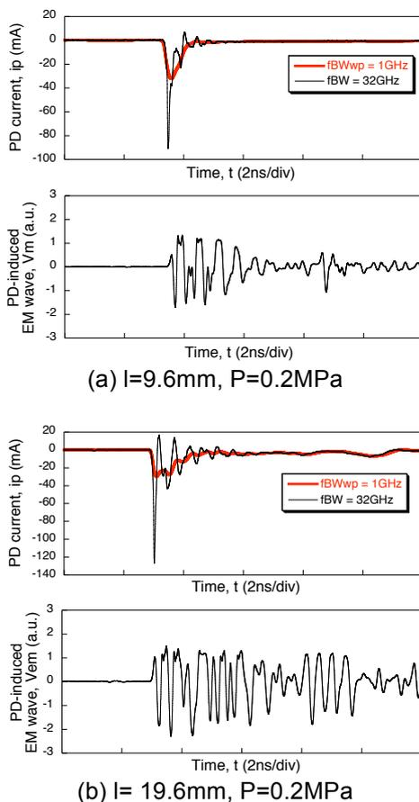
**Figure 11:** Simultaneous measurement of PD current pulse and the induced EM wave at different test conditions.
