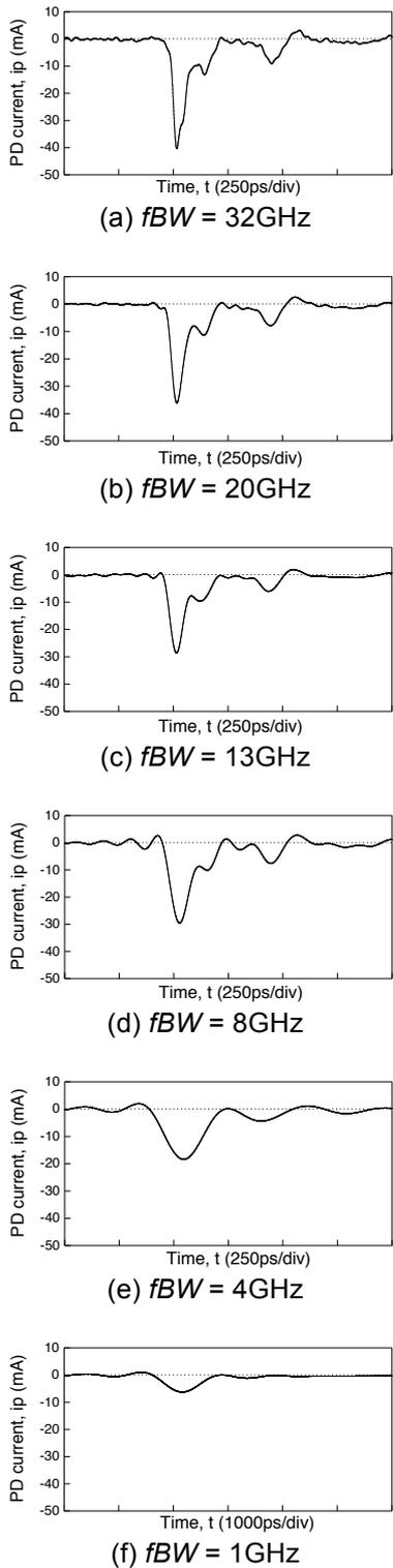
**Figure 2:** PD current waveforms in SF<sub>6</sub> gas measured with different frequency bandwidth *fBW* of the used oscilloscope (*l*=9.6mm, *P*=0.3MPa, negative corona).
