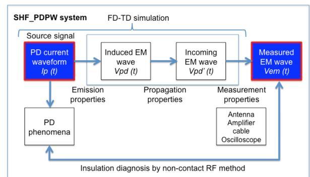
**Figure 10:** Schematic view of importance of the precise measurement of PD current pulse and the relation with the UHF method.
