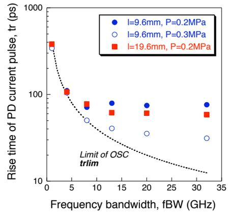
**Figure 9:** Relationship between the minimum rise time of the measured PD current pulses (Figure 3(b)) and the measurement limit of a rise time of the oscilloscope at each  $fBW$ .
