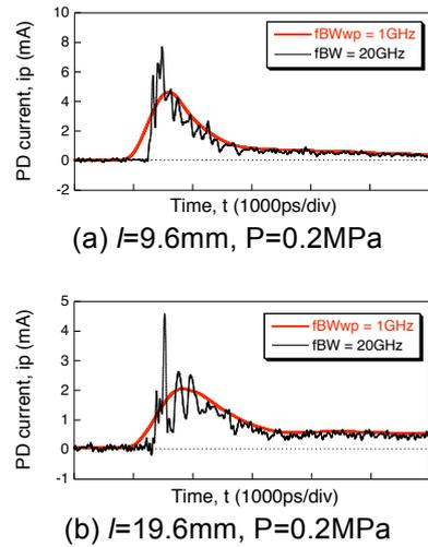
**Figure 6:** Typical examples of relationship between the measured PD current waveform with  $fBW=20\text{GHz}$  and the processed one with  $fBWwp = 1\text{GHz}$  at different conditions (positive corona).
