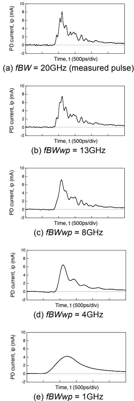
**Figure 5:** PD current waveforms processed by a function of the bandlimiting filter of the oscilloscope with the waveform processing frequency bandwidth  $fBWwp$  ( $l=9.6\text{mm}$ ,  $P=0.3\text{MPa}$ , positive corona).
