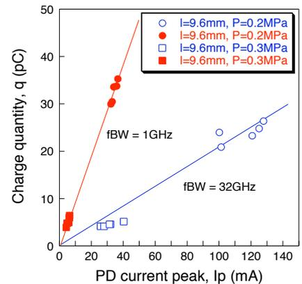
**Figure 4:** Relationship between *ip* and *q* of PD current waveforms measured with different frequency bandwidth *fBW* under different conditions (negative corona).
