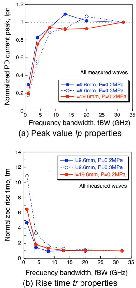
**Figure 3:** *fBW* dependences of normalized *ip* and *tr* of the measured PD current waveforms by the value at *fBW*=32GHz (negative corona).
