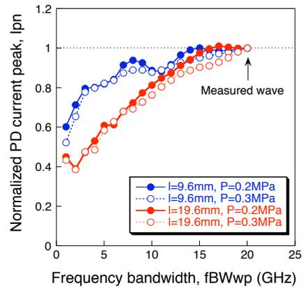
**Figure 7:**  $fBWwp$  dependence of normalized  $I_p$  of the processed PD current waveforms by the value at  $fBW = 20\text{GHz}$  (positive corona).
