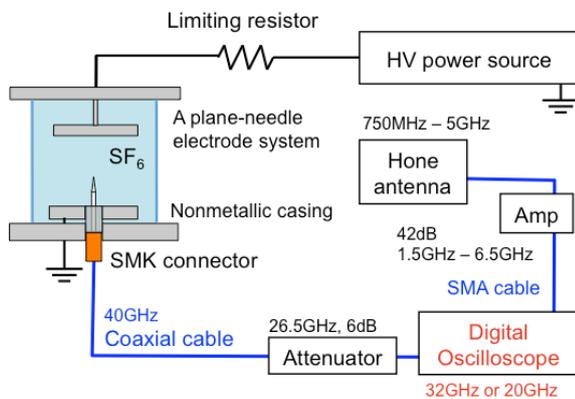
**Figure 1:** Experimental setup to precisely measure the waveform of PD current pulse in SF<sub>6</sub> gas with the SHF\_PDPW system.
